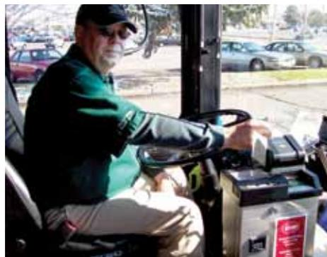
The new boxes greatly enhance ease-of-use and convenience for transit riders by enabling them to pay their bus fare with a quick swipe of a card versus waiting to have an old punch-pass punched or other pass checked by the driver. The change counter also speeds fare collection by eradicating the arduous process of change counting for passengers and drivers alike.
