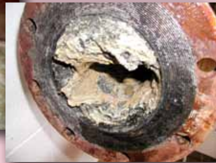
Above: Chunks of grease that arrived at the wastewater treatment plant.
